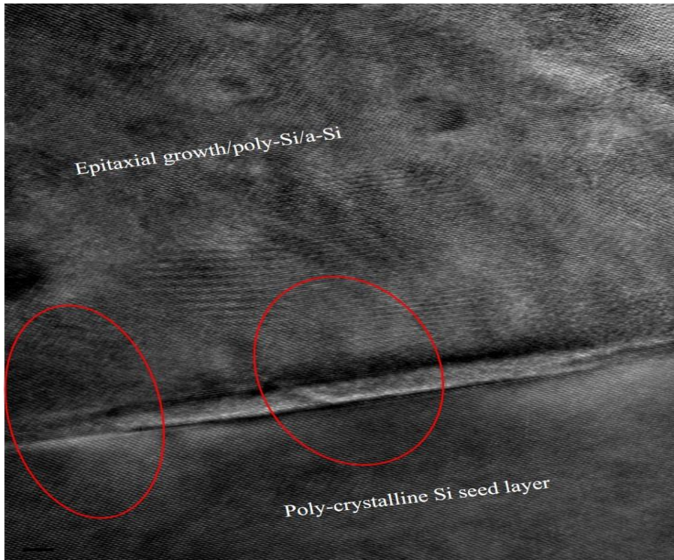
Figure 59. TEM image for epitaxial growth of Si on AIC seed layer.
