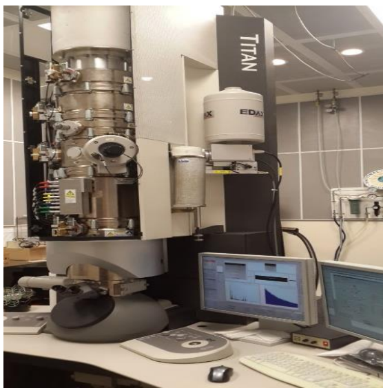
Figure 21. FEI Titan HRTEM that was used in this research (picture taken by the author).
