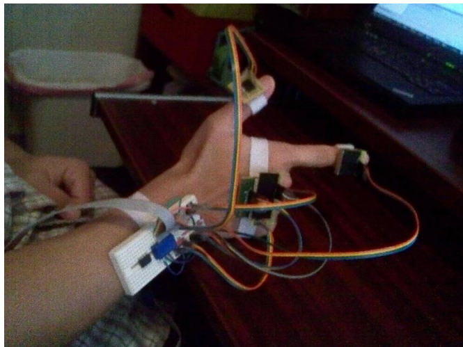
Figure 2.2 – Accelerometer based Hand pattern recognition [16]
