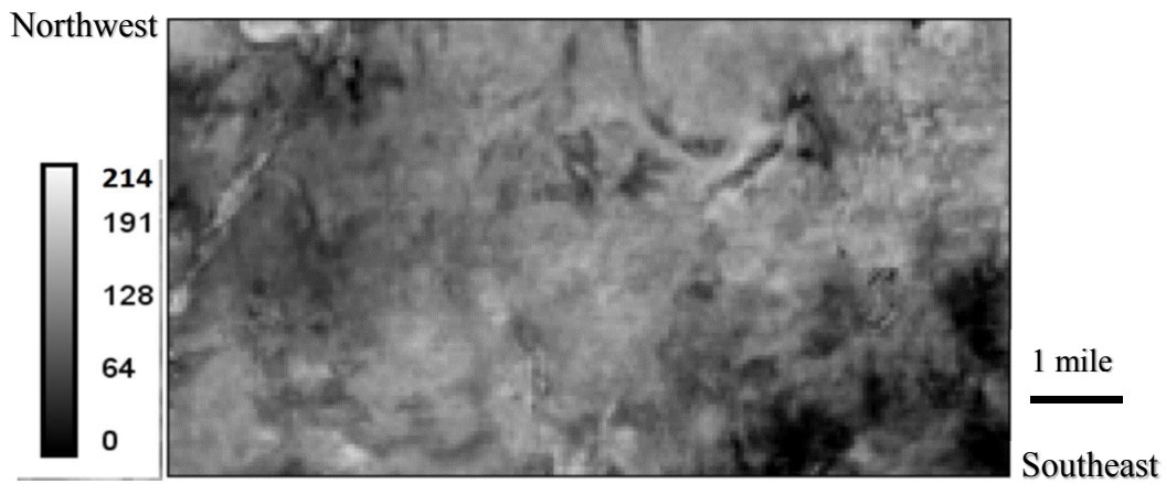
Figure 6: Amplitude structure of the middle of the Mississippian Formation. For the model this image represents the area at 150 feet within the model block. (Seismic time-depth 620ms.)
