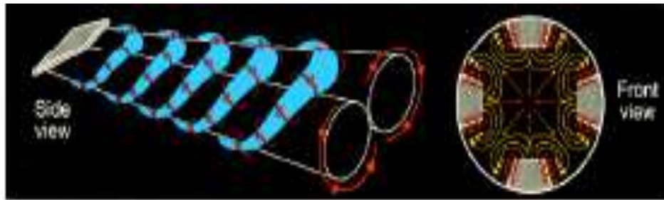
Figure 8 : Hairpin and longitudinal vortices caused by tabs (7)
