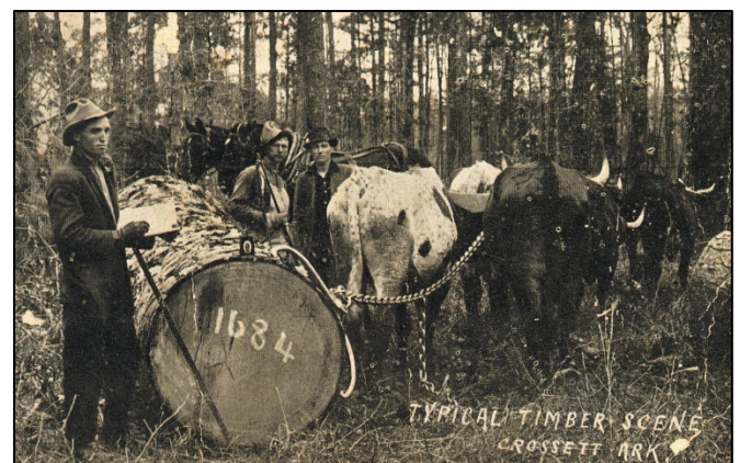
Figure 1. A pine log from Ashley County, Arkansas, with the quantity of lumber estimated to be sawn from this log written on the photograph (1,684 board feet). Copy of a historical postcard courtesy of the Crossett Public Library.
