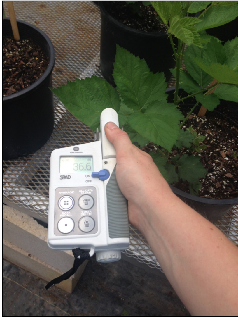
Figure 4. Estimated leaf chlorophyll content measured as measured by Minolta SPAD-502 Plus® monitor of 'Prime-Ark® 45' blackberry grown in pots as affected by four shade treatments, 2014, Fayetteville, AR.
