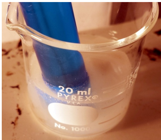
Figure 4. Oxygen bubbles emerging from the photoirradiated heterogeneous mixture: water and SiO 2 -TiO 2 -Zn- o -TCPP.
