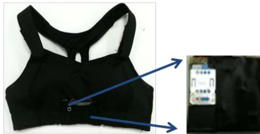
Figure 14. Exterior of the transmission module of the E-Bra system
