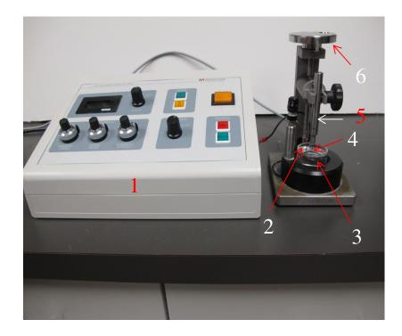
Figure 2.2: Submerged experimental electrochemical etching setup: omicron DC power supply (1), copper wire with its ring (2), electrolyte solution in the glass beaker (3), tungsten wire (4), magnetic metallic cylinder (5), and micrometer screw (6)
