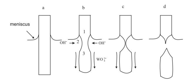
Figure 2.4: Schematic sequences of the etching mechanism. a) shows the formation of initial electrolyte meniscus. b) and c) illustrate the flow of tungstate ions  $(WO_4^{2-})$  down the sides of W wire and OH<sup>-</sup> towards the neck of the wire. d) shows the lower part drops off.
