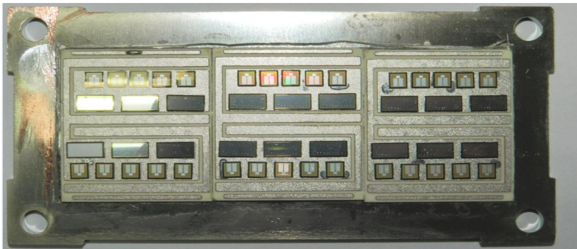
Figure 3.20: Fabricated power module.
