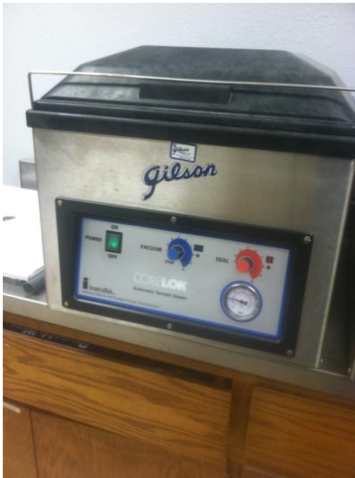
Figure 3:8: Corelok ® Machine and Sealed Sample
