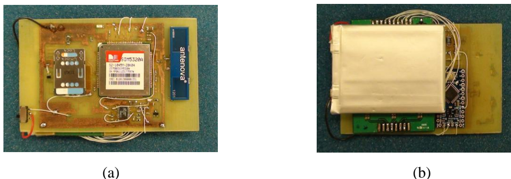
Figure 4.12 Images of the wireless HST system with GSM/WCDMA; (a) top and (b) bottom side of the system
