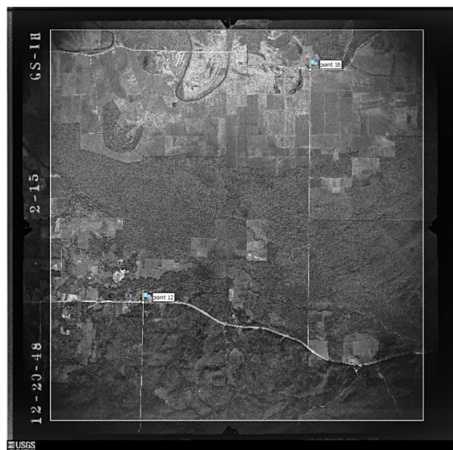
Figure 2 Sample Single Frame (USGS, AR1IH0000020015) with mask excluding the edges of the film, labels, and fiducials. GCPs are shown as blue numbered flags.
