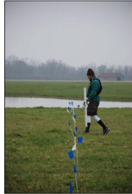
Figure 6.4. Pin flag method using the Grad 601. Photo taken by Anthony Clay Newton.
