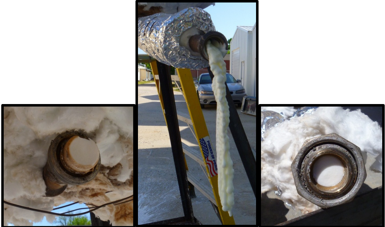
Figure 67: Salt Frozen in Lines during Testing
