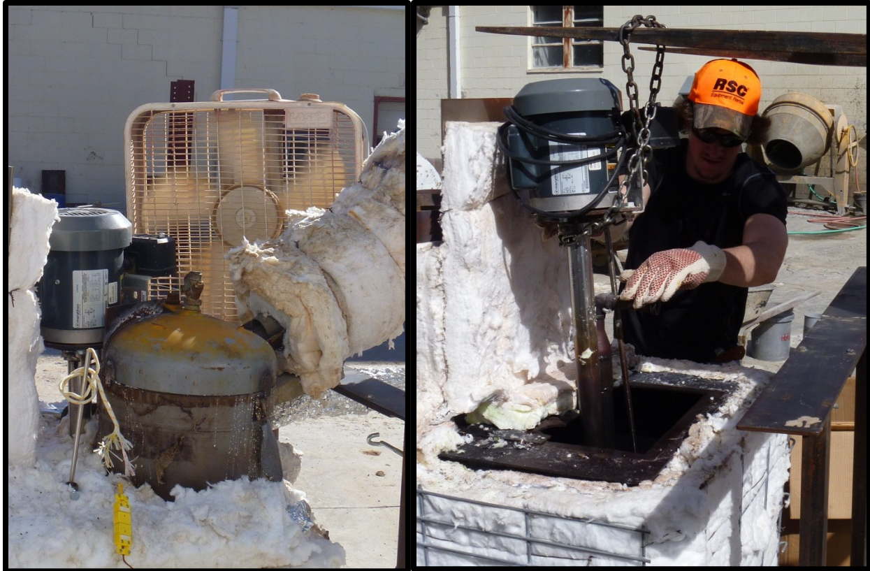
Figure 69: Motor Driving Pumping Unit During Testing (Left) and Pumping Unit Being Removed to Allow Replacement of First Motor (Right)
