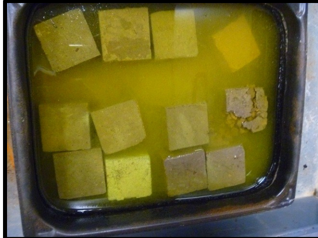
Figure 47: Concrete Specimens in Molten Salt Bath (John, 2012)
