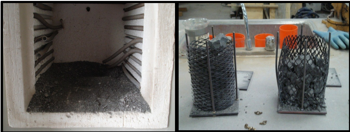
Figure 46: Oven Damaged While Heating Concrete Specimen (Left) and Cylinder Cage Damaged While Heating Specimen (Right) (John, 2012)
