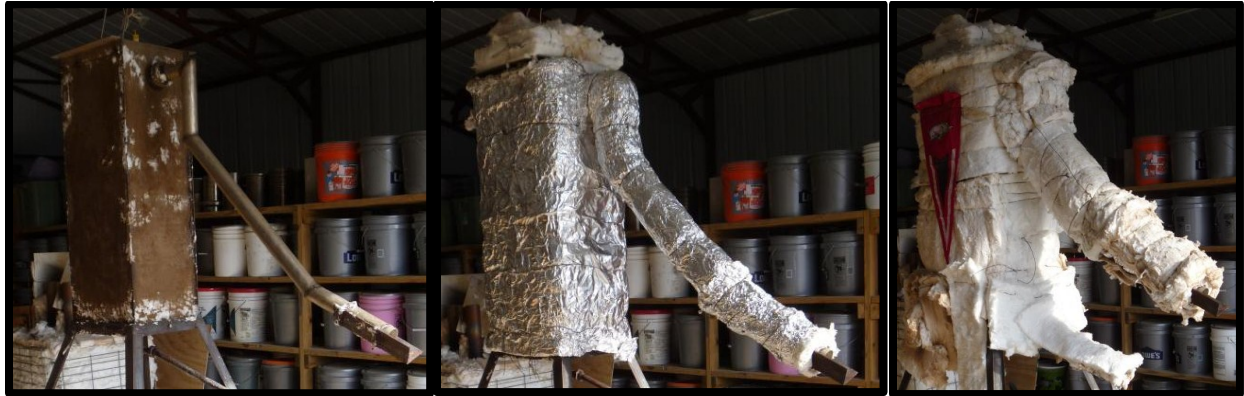
Figure 49: Thermocline Tank: Un-insulated (Left), One Layer of Insulation and Aluminum Foil (Middle), and Two Layers of Insulation (Right)
