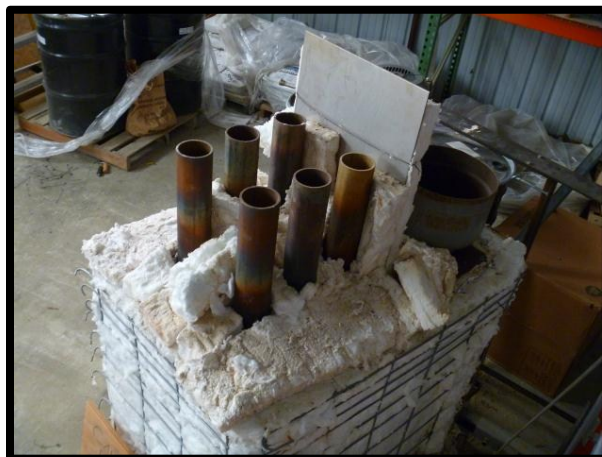
Figure 50: Insulated Salt Storage Tank
