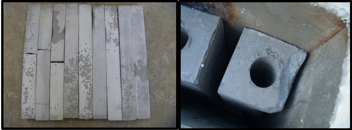
Figure 70: Spalling Damage to TC1000 Concrete Specimens
