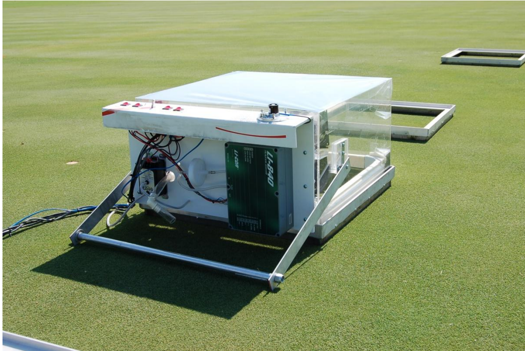
Figure 2. Infrared gas analyzer attached to the PVC shield to reduce sunlight and heat to the gas analyzer.
