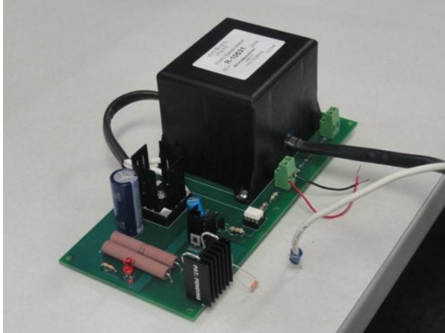
Fig. 4.12. SiC SGTO turn-on gate driver from [84].
