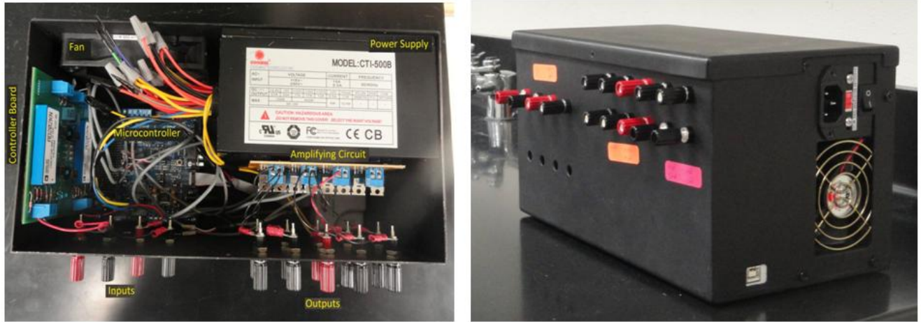
Fig. 4.30. Inside and outside of SSFCL controller box.
