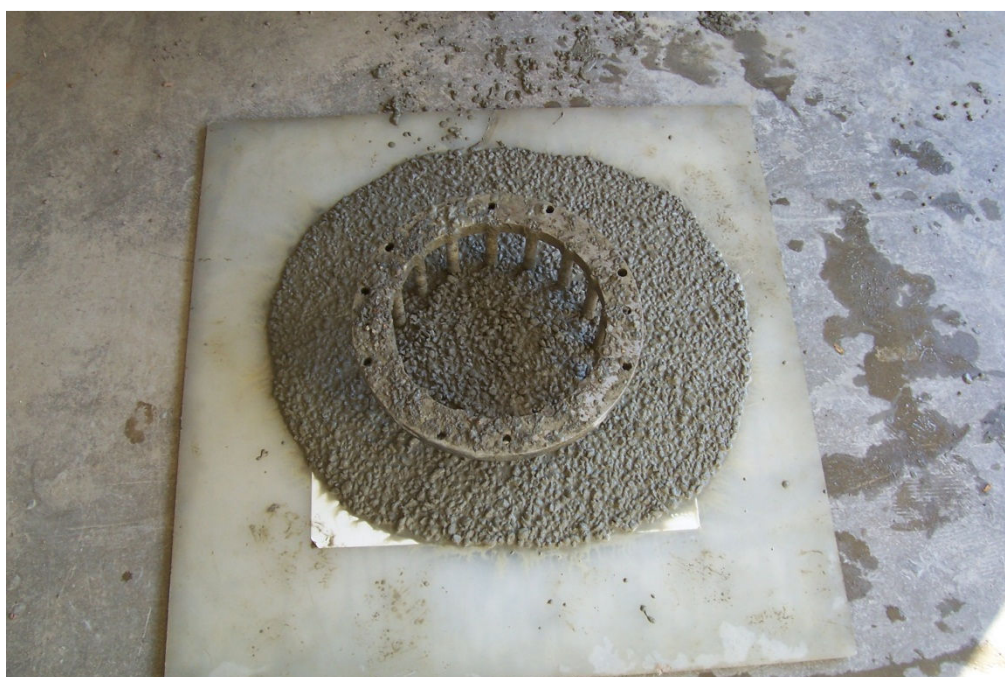
Figure 3.10 J-Ring Test Part 2: Measure the Flow
