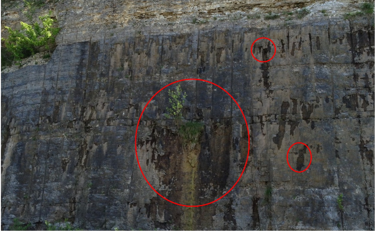
Figure 34 – Outcrop exposure of the Reeds Spring exhibiting an example of fluid permeability pathways and conduits through bedding planes and fractures shortly after rainfall. The red circles highlight a couple areas where fluid outpour can be identified to different scales. This exposure is located on Hwy 412, outside Pedro, AR.
