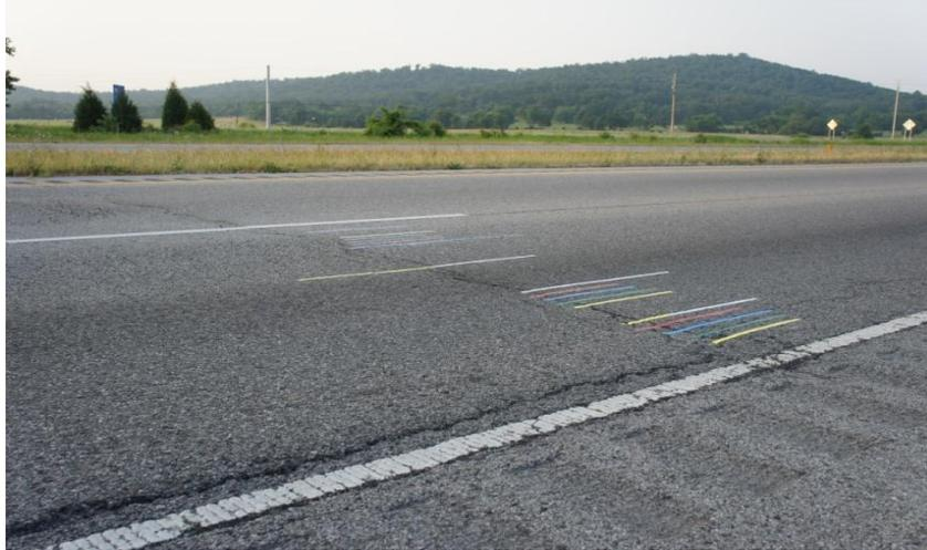
**Figure 18 Mark of reference lines in the field**
