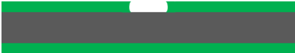
Figure 8: Side view of after the chemical etching process
