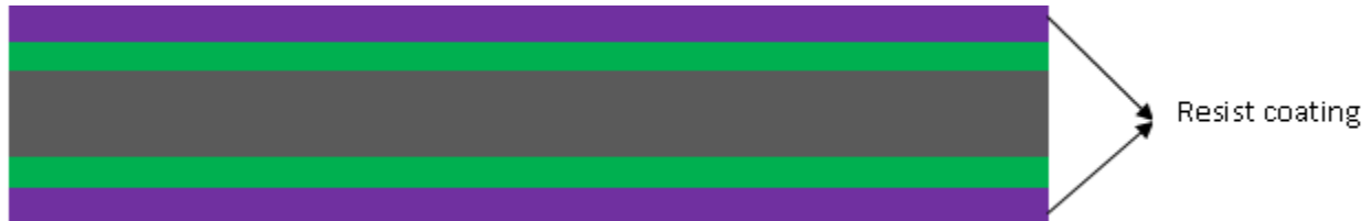
Figure 4: Wafer with layer of resist coating on both sides
