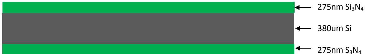
Figure 3: Side view of Silicon wafer with Si_3N_4 deposited on both sides
