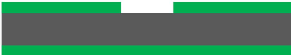
Figure 9: Side view of wafer after the RIE Process is complete
