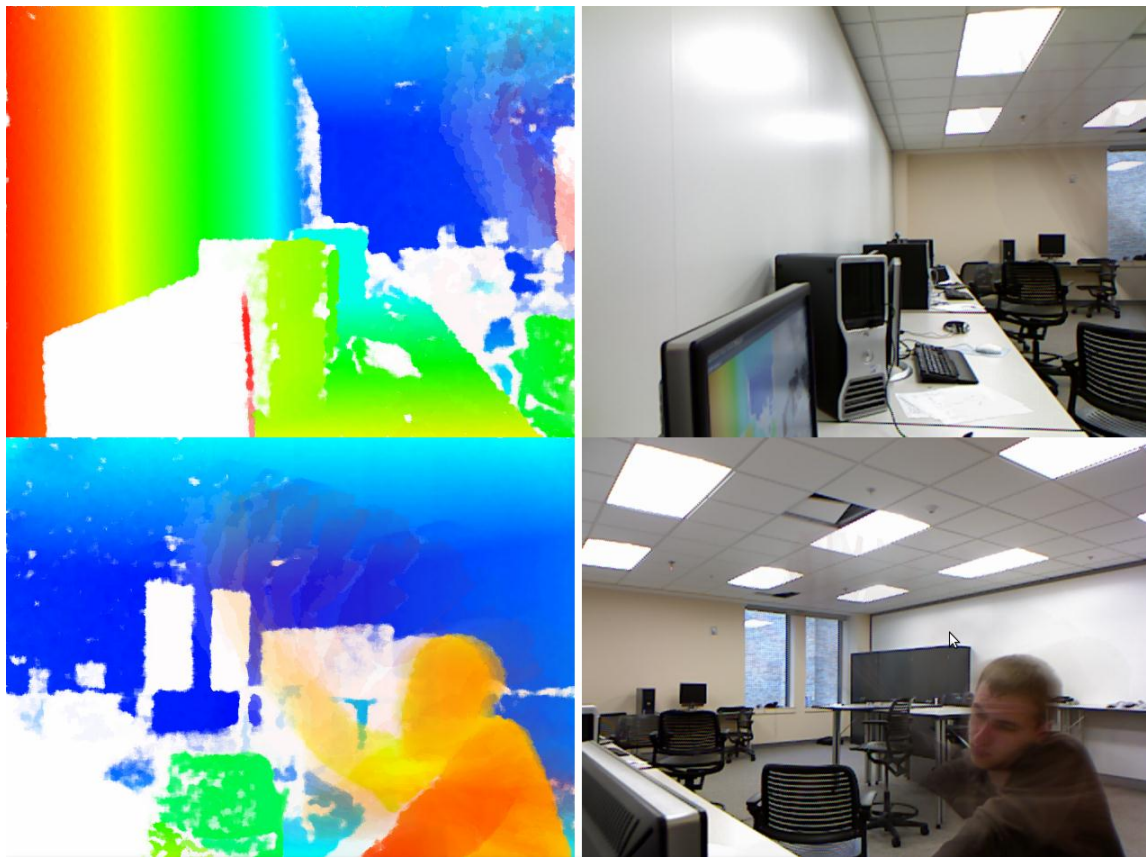
Figure 9: Infinite impulse response averaging with 10% of the new image and 90% of the average.
