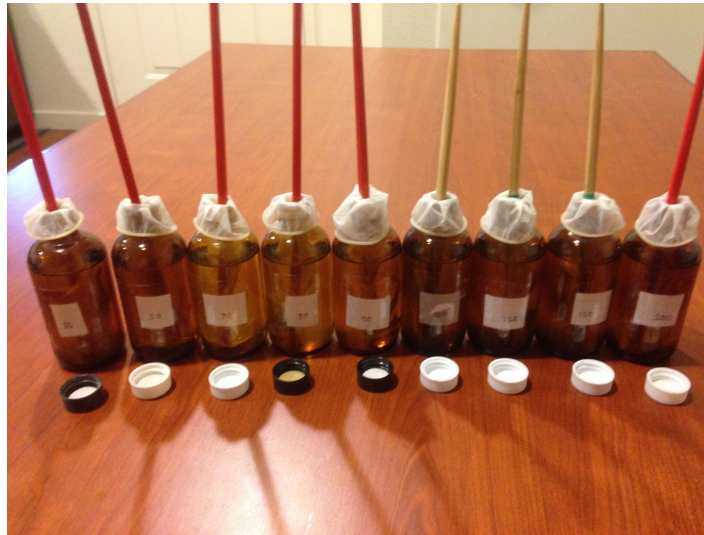
Figure 3-8: Glucose solutions in glass bottles. Arranged left to right; 30, 50, 70, 80, 90, 100, 125, 150, 200 mg/dL
