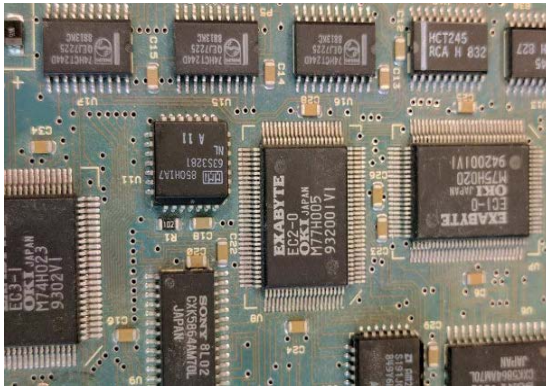
Figure 1: Typical circuit board with surface-mounted integrated circuits or chips.
