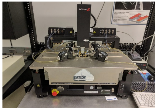
Figure 14: Wafer probe station used for preliminary electrical evaluation of our samples. This instrument features four-point probe capabilities, an optical microscope for precision measurements, and a pneumatic cushioning and vacuum system for stability.
