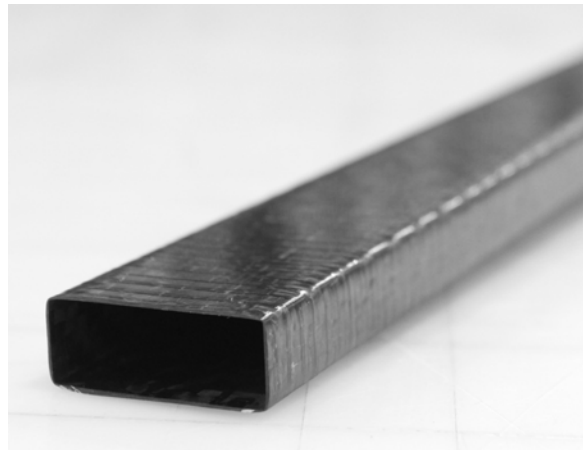
Figure 3.4: Isometric view of the 0.375” x 1” cross-section of the carbon fiber tubing 10
