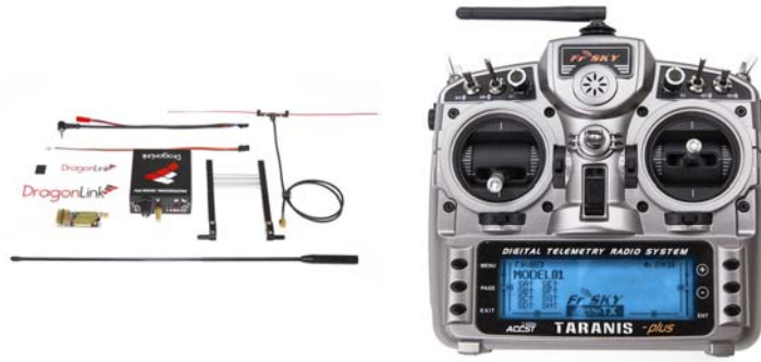
Figure 3.12: Dragonlink setup for long distance communication between the taranis radio controller (shown on the right) and flight controller 17
