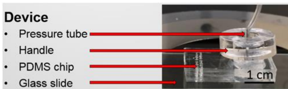
Figure 2.4.1.2: Direct view of chip setup. Highlighted is the pressure inlet, handle, chip, and glass substrate.
