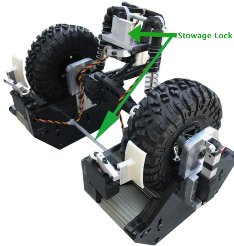
Figure 3.17: VDV prototype photograph with stowage lock call-out
