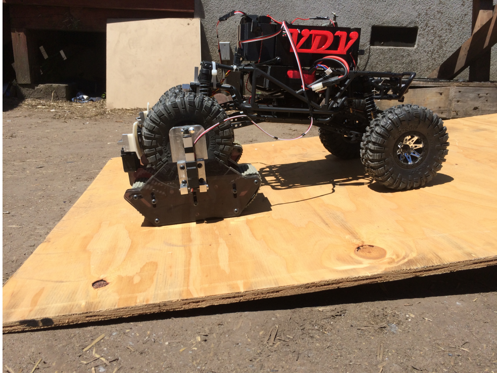
Figure 4.26: VDV traveling up 5 degree slope in track mode.
