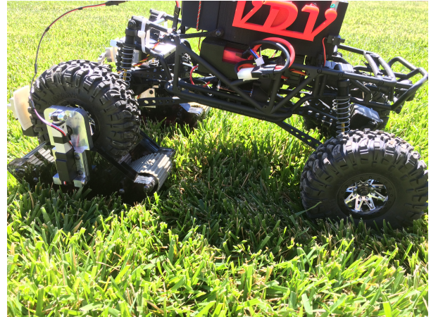
Figure 4.25: Tracks sinking in grass.
