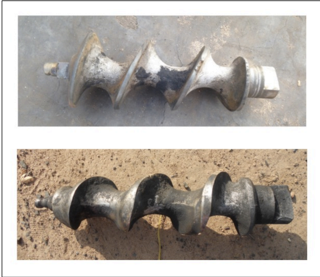
Figure 1 - A new AEST auger (top) and a twice-repaired auger (bottom), reproduced with permission [2].
