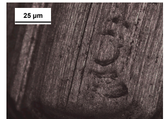
Example of pockmarks on heat-treated sample H7, 5x
