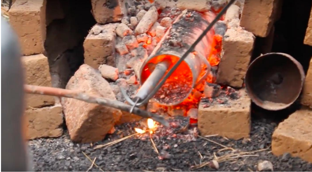
Figure 31 - The auger is removed from the kiln using sticks and metal rods, reproduced with permission [15].
