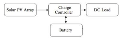
Figure 23: Flowchart of Stand-Alone PV System<sup>7</sup>
