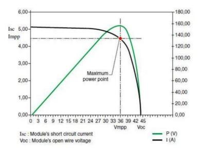
Figure 26: Typical IV Curve of a Solar Panel Showing MPP
