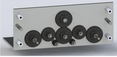
Figure 15: Rendered image of internal gear train
