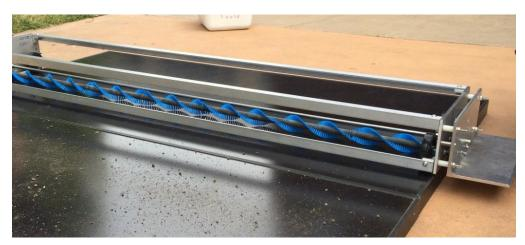
Figure 11: The Selected Brush Design Installed on Prototype
