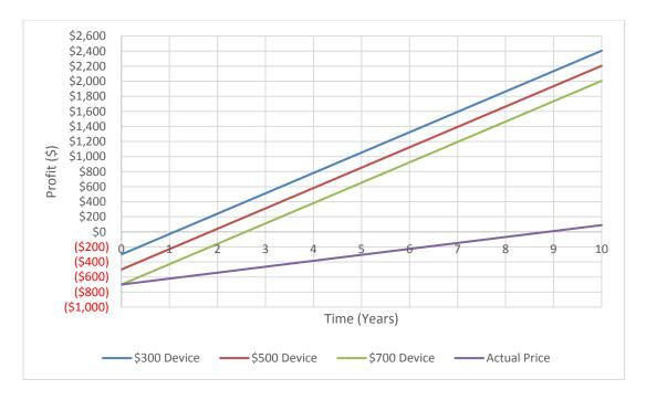
Figure 45: Break-even analysis including the actual price and efficiency of the device
