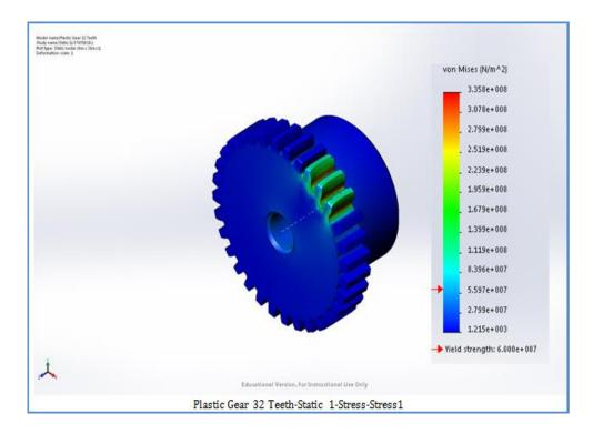
Figure 19: Solidworks FE spur gear stress analysis
