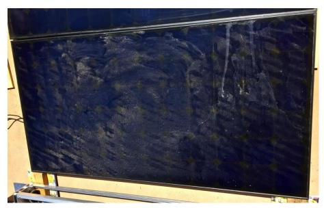
Figure 29: Dirty Panel after four Passes by System
