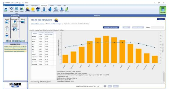
Figure 35: Homer model architecture and annual global horizontal irradiance used for simulation<sup>9</sup>
