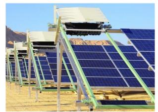
*Figure 5: Ecoppia E4 cleaning system*<sup>7</sup>(*Reproduced without permission*)
