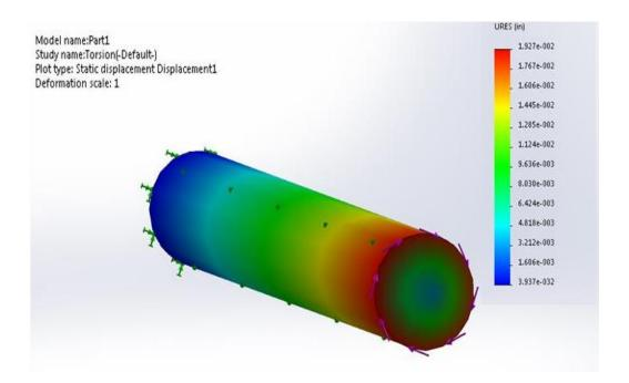
Figure 17: Solidworks FE driveshaft displacement analysis
