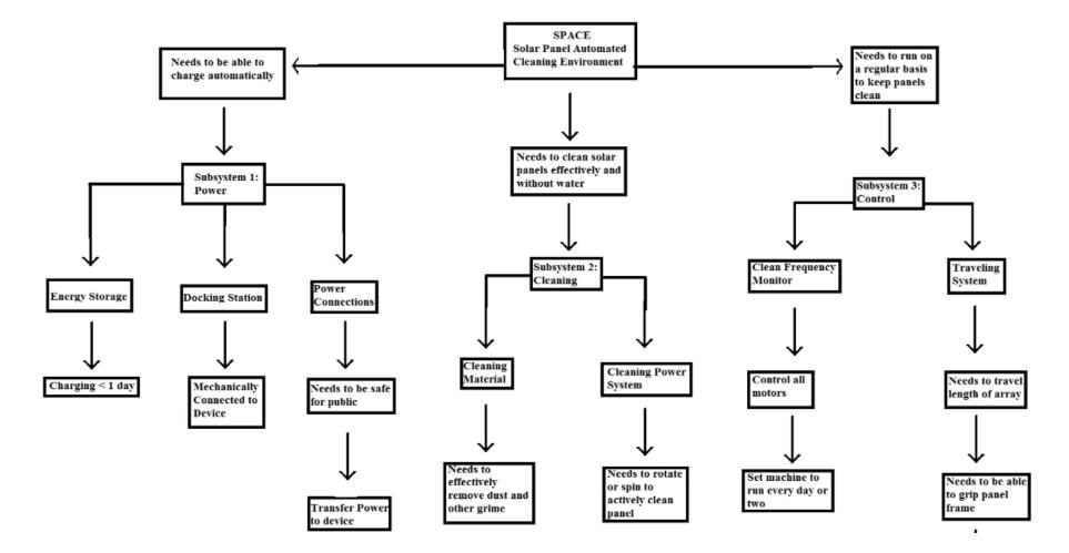
Figure 10: Layout of the system level design with main subsystems
