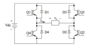
Figure 22: Diagram of a H-Bridge Detailing the Four Different Transistors
