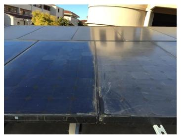
Figure 1: Cleaned panel (left) vs. Soiled panel (right) (Team Photo)
