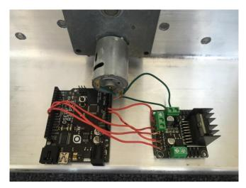
Figure 20: Control system hardware overview
