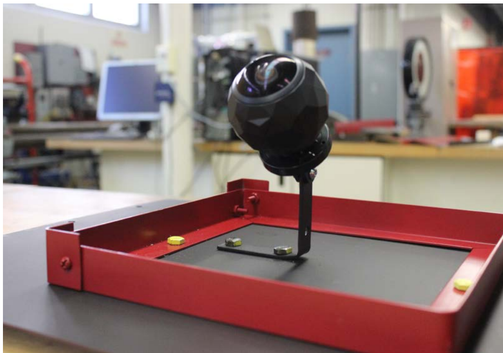
Figure 3.4: 360Fly Camera mounted on top of the chassis on SAFER.
