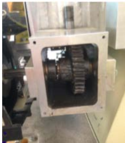
Figure 5.1: The existing gearbox with the exposed gears, posing a safety risk.
