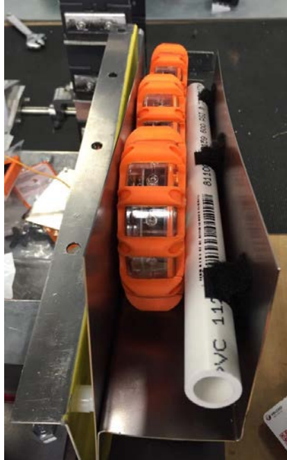
Figure 3.9: Beacons loaded up in the dispenser. The PVC pipe supports the beacons so they can exit the dispenser smoothly and consistently.
