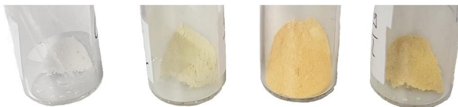
Figure 5.24: Photograph of the different undoped and Sn-doped CsTaWO 6 samples. From left to right: undoped CsTaWO 6 nanoparticles, Sn-doped CsTaWO 6 via SSR and Sn-doped CsTaWO 6 nanoparticles for 1 d or 7 d (rightmost).
