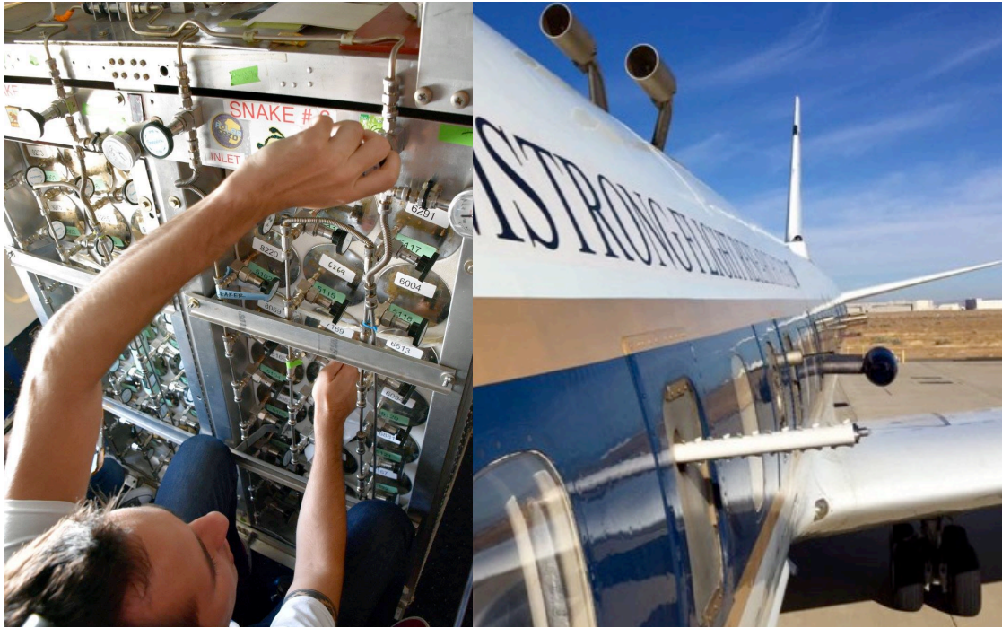
Figure 4. UCI Whole Air Sampler instrument onboard the DC-8 aircraft (left) and a view of the modified DC-8 with intake probes (right).
