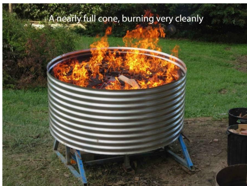
Figure 10. Kon Tiki kiln with flame curtain. Source: www.thebiocharrevolution.com/blog/biochar-production-in-kon-tiki-australia-1
