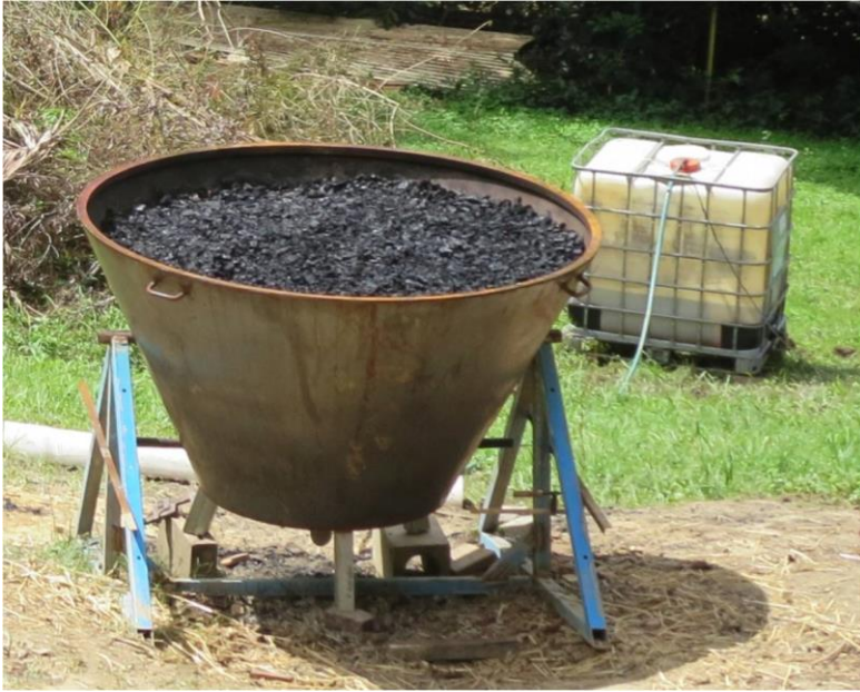
Figure 9. Kon Tiki kiln. Source: www.thebiocharrevolution.com/blog/biochar-production-in-kon-tiki-australia-1
