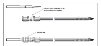
FIGURE 1 | Representation of soil probe design used to sample volatiles belowground. Probe is inserted into soil and connected to a vacuum pump. Reprint from "Extending explorations of belowground herbivore-induced plant volatiles: attracting natural enemies of root pests in multiple contexts (Ali et al., 2012).
