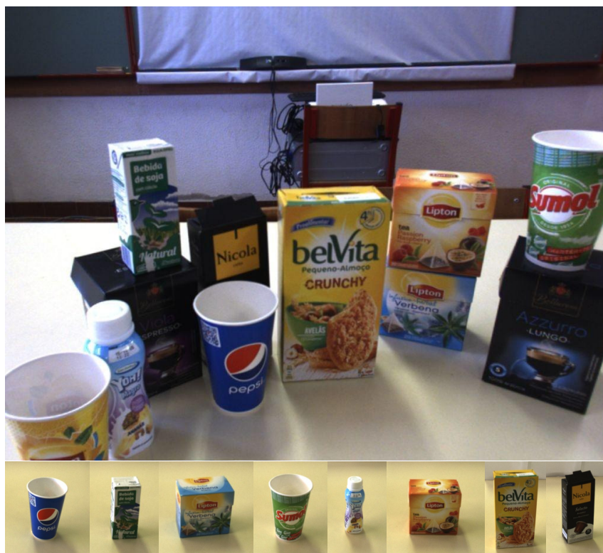
Figure 4.13: More examples of the robot recognizing objects. The recognized objects are shown below the image. Since the yellow cup is only partially visible in the bottom left corner of the image, it could not be recognized. The two black boxes were also not recognized because they generate only a very small number of keypoints, making it hard to recognize them.
