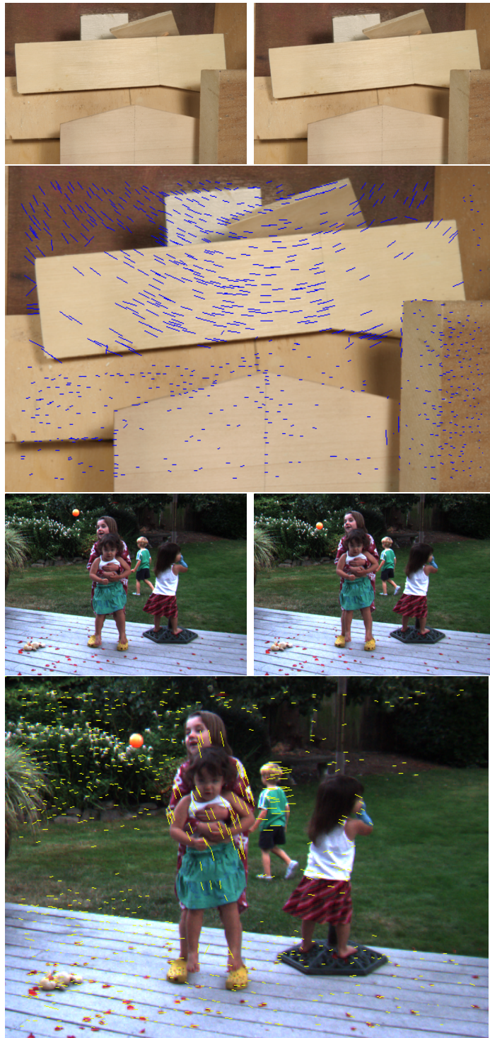
Figure 3.11: Example of optical flow determination using our keypoints and keypoint descriptors. Rows 1 and 3 show two sequential frames from two different sets. Rows 2 and 4 show the optical flow results obtained from matching keypoints between the two frames. The images belong to the Middlebury Optical Flow dataset [Scharstein, 2009a].
