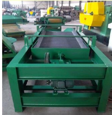
Figura 14. Pantalla vibradora secundaria ( vice vibrating screen )
