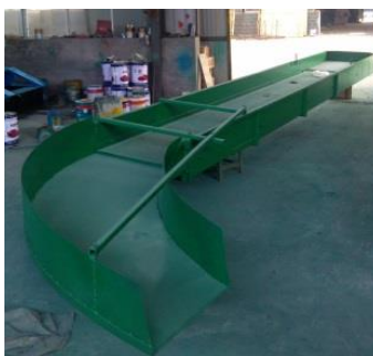
Figura 13. Pantalla vibradora principal (main vibrating screen)
