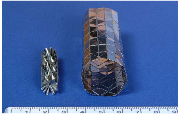
Figure.1.8: Cylindrical tube with 0.5 mm width folds in its fully folded and expanded configurations [1.30]
