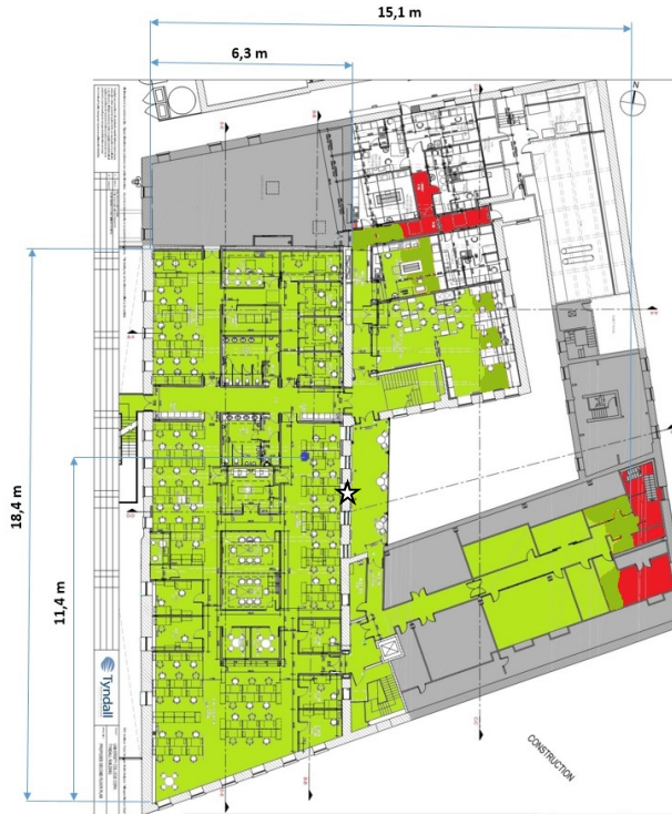
Figure 12. 868MHz range test after compensation
