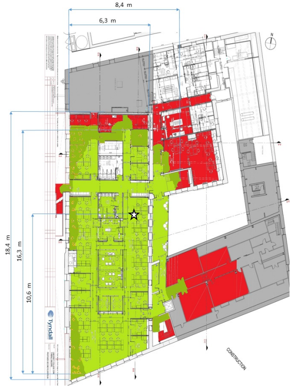
Figure 10. ZigBee 2.4GHz range test
