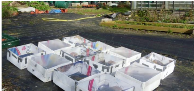
Figure 4.2(a) Outdoor experimental setup 50x50cm corri-board frames, were used to mount the filters. These were tilted slightly at the northern edge
