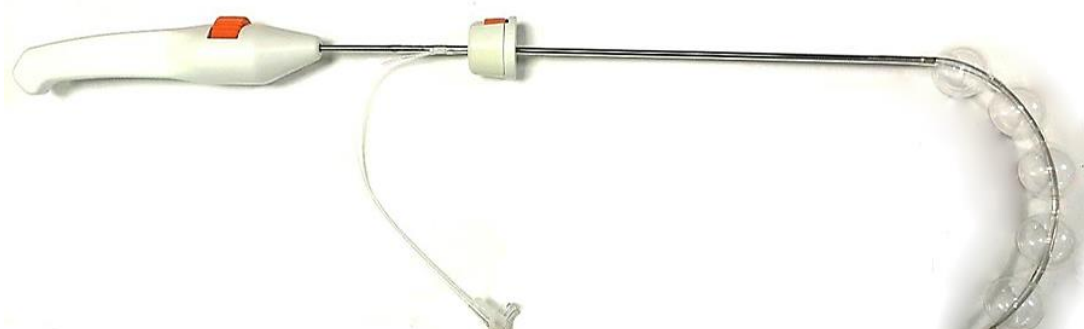
Figure 3.7 Retractor prototype pictured in its inflated, curved position with non-return inflation valve.
