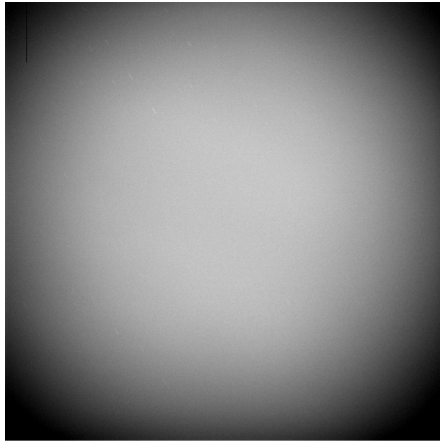
Figure 2.2: Flat field image taken from the C2PU telescope, which shows how vignetting affects the image.
