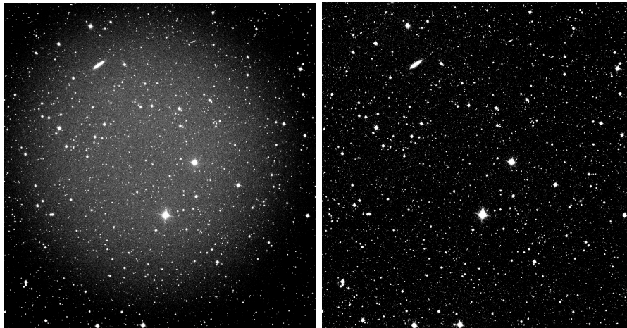
Figure 2.1: An example of the difference between a raw and a reduced science image. The left shows a typical raw image taken using the CCD on the 1m C2PU telescope, while the right shows the same image after bias subtraction and flat fielding.
