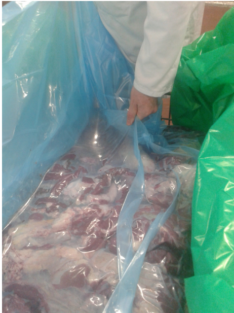
Fig. 4.15 Photo demonstrating vacuum pulled on bin.
