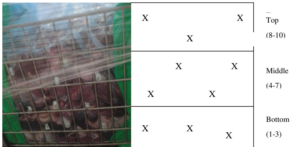
Fig. 4.14 Orientation of sensors on bin
