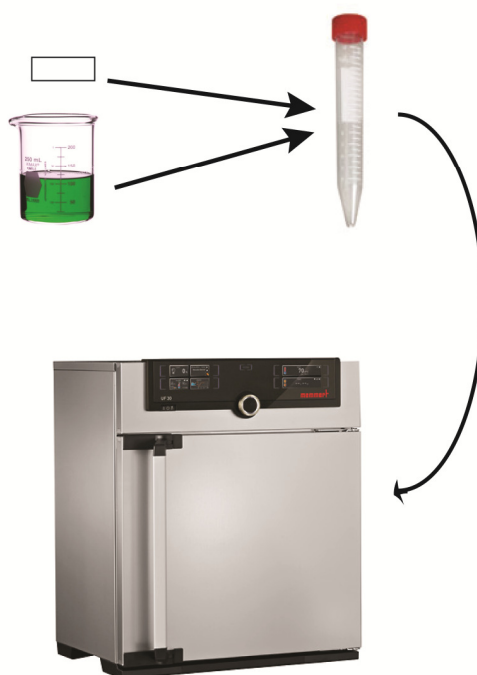
Fig. 3.7 Diagram showing swelling method. Fabric strip and dye/solvent cocktail are placed in plastic vial and incubated in oven at 65 °C for 1 h.
