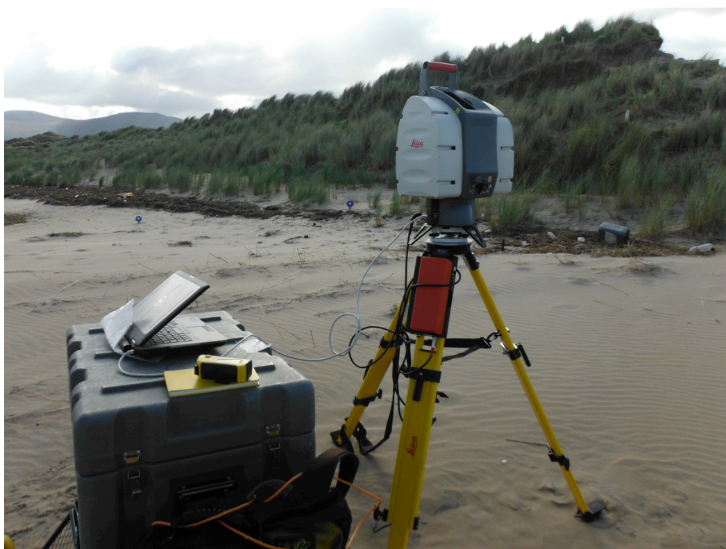
Figure 7.9 Leica ScanStation setup at Rossbehy field site. Looking north at main dune barrier terminus. Source: author's own (15 November 2012)
