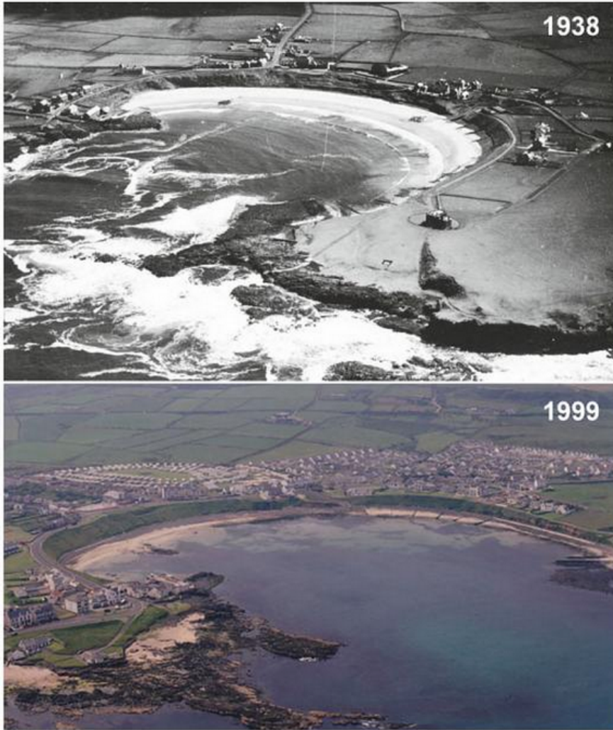
Figure 4.6 Oblique aerial photos of Portballintrae Beach in 1938 (top) and 1999 (bottom) illustrating beach narrowing as a result of the installation of a pier in its western section. Source: Jackson (2012)
