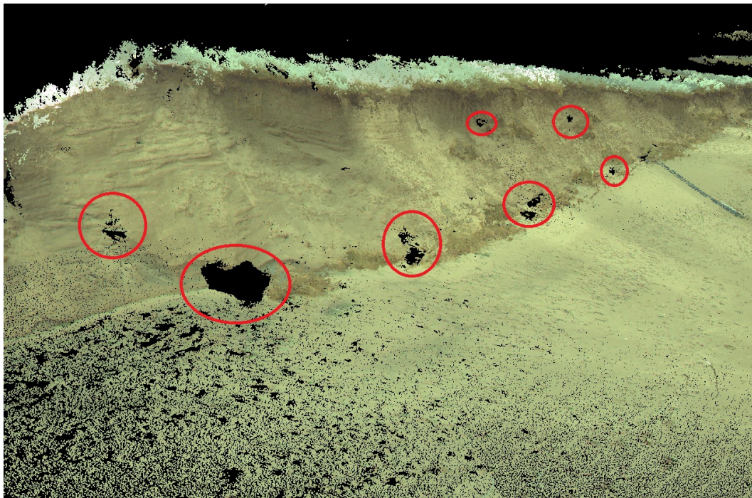
Figure 6.4 Shadow zones - zones of missing data located behind obstructions to the laser scanners field of view, resulting in 'gaps' in the point cloud. These can be minimised by obtaining multiple surveys over the same area from different angles. Source: author's own data obtained at Rossbehy field site
