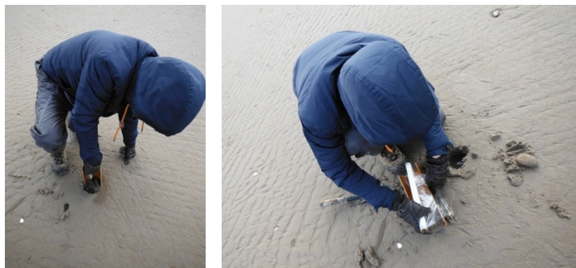
Figure 9.5 Sampling with half pipes and trowel.
