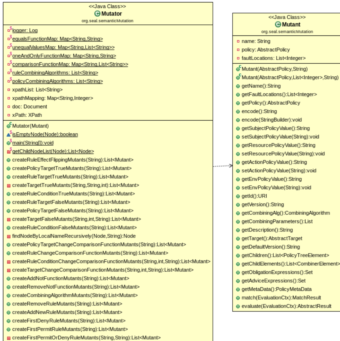
Figure 5.5 UML Class Diagram of Component Mutation
