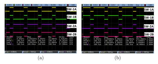
Figure 6.3: (a) IGBT gate driving signals at D = 0.25 (b) IGBT gate driving signals at D = 0.75.
