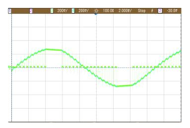
Figure 6.8: Current through the top switch when duty cycle D = 0.5.
