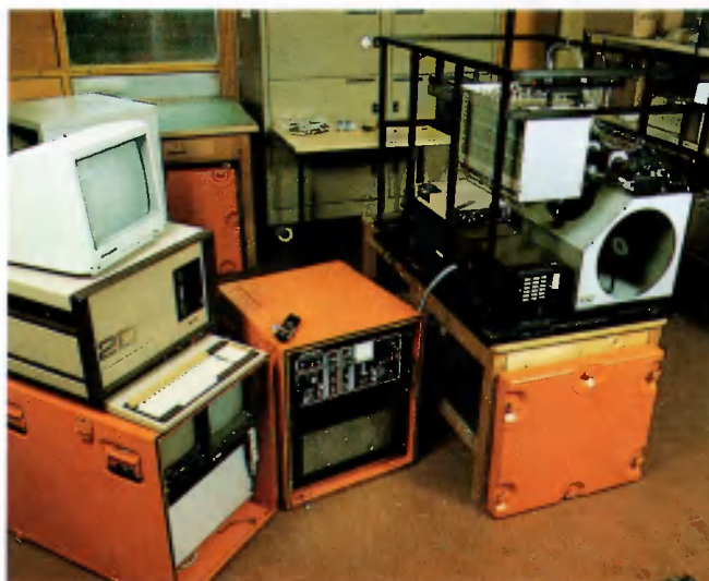
Fig. 16: The "Time Resolved Lidar Fluorosensor" under construction at CISE S.p.A. (Milano). The top right structure contains the laser, the telescope and the streak camera.
