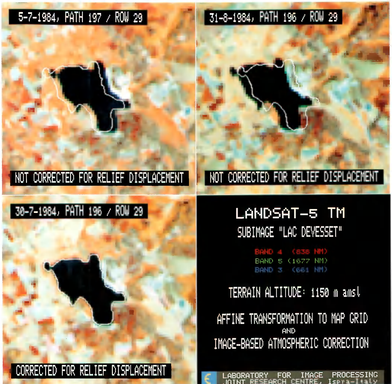
Fig. 2: Correction of relief induced distortions on the localisation of a lake (altitude 1150 m). The white contour corresponds to the exact topographic location. The displacement occurs to the right or to the left when the satellite is viewing from the West or from the East.
