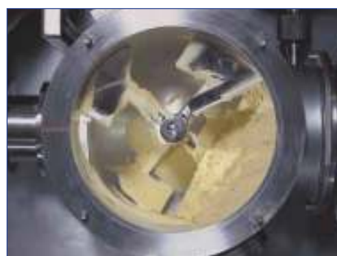
A dry mixing technique is applied for processing GMO reference materials to avoid DNA degradation
