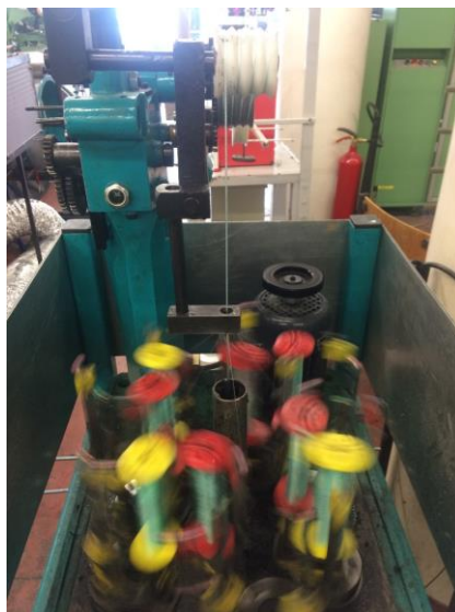
Figure 11- Vertical braided machine used in the development of stents.
