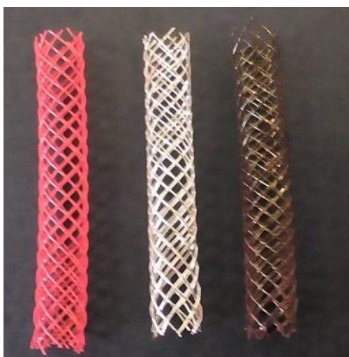
Figure 52 -Braided PES stents uncoated, and coated with Ag and AgO100, by the same order.
