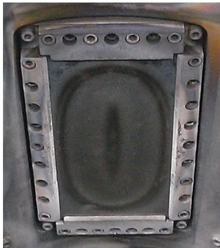
Figure 10- Example of a target used in magnetron sputtering.
