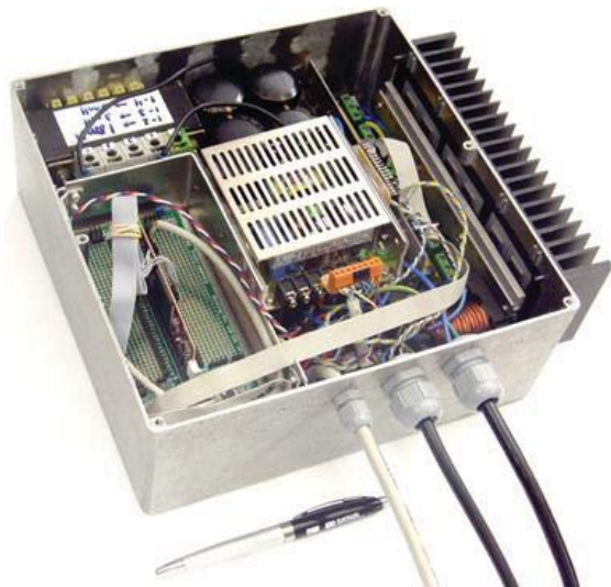
Figure 2: Reconfigurable laboratorial prototype of the on-board EV battery charger used to obtain the experimental results.
