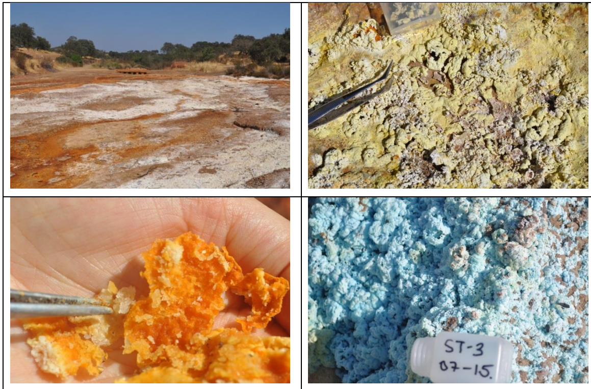
Figure 1 Field images showing the occurrence modes of typical efflorescences, composed by aluminium and magnesium sulfates. a) General view of Meca River with white powder efflorescences; b) crustified efflorescences dominated by aluminocopiapite ; c) Orange plate efflorescences dominated by magnesium sulfates (epsomite); d) Blue-green globular efflorescences with magnesium sulfates (hexahydrate) and copper sulfates (chalchantite).
